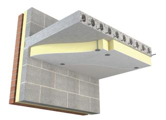
**3.** Using XtroLiner Soffit Plus on soffit areas, whether new build or refurbishment situations, provides the most efficient U-Values with minimal thickness of insulation. The product achieves a thermal conductivity of 0.021 W/mK and has a Euroclass B fire classification.
